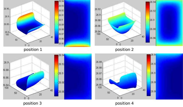
different placement locations for the device. The temperature achieved for every register in the register file is a factor of the number of accesses to the register, the temperature reached by the neighboring registers, and the thermal transfer promoted by the hot functional units close to the register file. All these parameters are considered by the thermal model to characterize the temperature profile.
