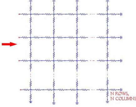
Now, from Figure 3, the circuit can be decomposed in a matrix of  $N$  rows by  $M$  columns of registers, and the resistance of every row can be calculated as follows.
